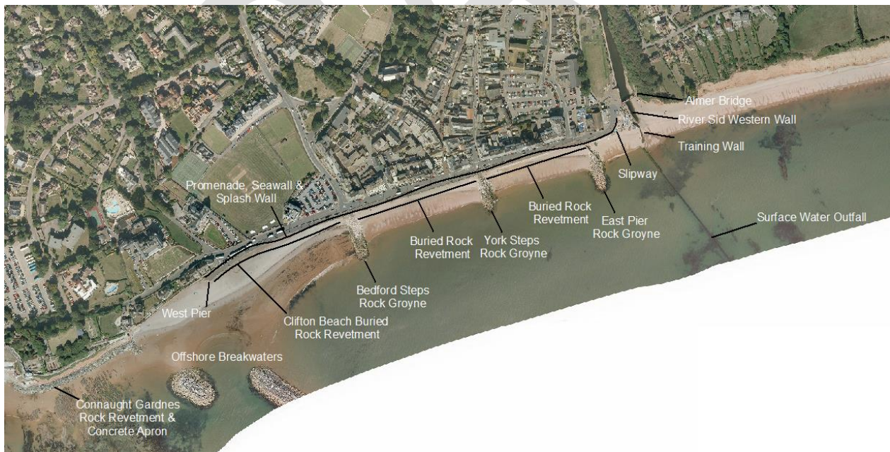
Figure 1-3: Sidmouth's current coastal defence arrangement
