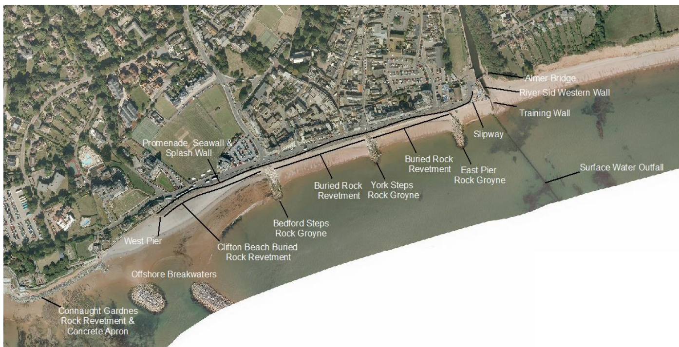
Figure 6: Sidmouth's current coastal defence arrangement.
